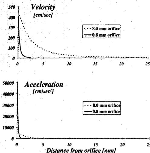
**Figure 2.** Effect of orifice size on the instantaneous acceleration. Although peak axial centerline velocity is similar for both the 0.8-mm and the 8.0-mm orifice, maximal acceleration is much higher for the smaller orifice, scaling approximately inversely with the orifice diameters.
