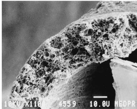
**Figure 5.** Electron micrographs of high molecular weight poly-L-lactic acid-dexamethasone stent coatings before (**top**,  $\times 1,000$  [reduced by 30%]) and 28 days after implantation (**bottom**,  $\times 1,100$  [reduced by 30%]) in porcine coronary arteries. Dexamethasone crystals visible before elution (**arrow**) are no longer present after 28 days, although polymer matrix appears largely intact.
