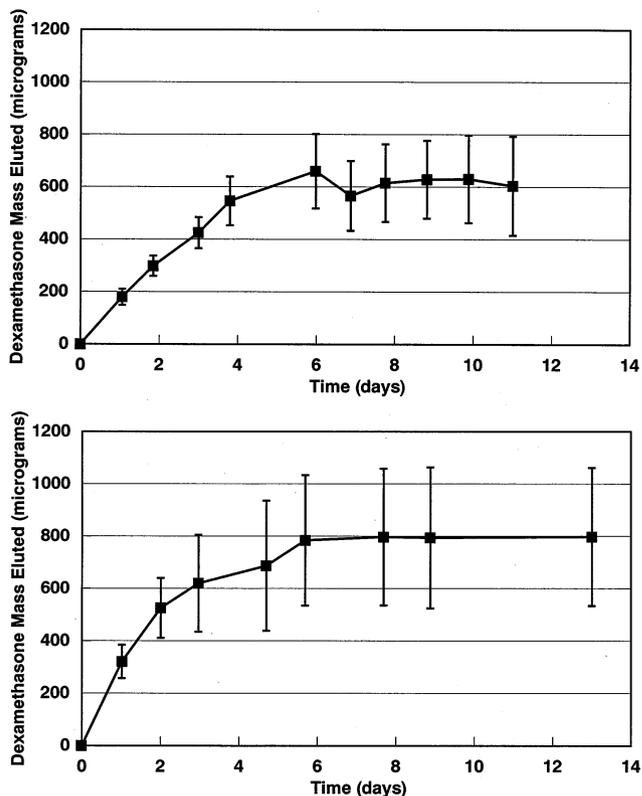
**Figure 3.** Cumulative (mean ± SD) in vitro dexamethasone elution from poly-L-lactic acid (PLLA)-dexamethasone-coated stents over 12-day period. **Top,** Low molecular weight PLLA (three stents). **Bottom,** High molecular weight PLLA (five stents).
