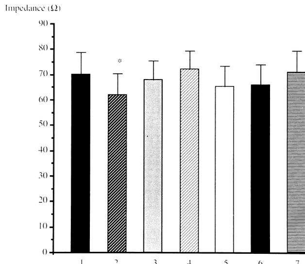
**Figure 3.** Mean ED50% and standard deviation for impedance for all seven lead configurations. \* $p \leq 0.05$ , configuration 2 versus configuration 4.
