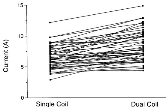
**Figure 2.** Peak current at defibrillation threshold. The results from each of the 50 patients are shown for the single- and dual-coil lead configurations. Note the consistent reduction in peak current with the single-coil configuration despite increased energy requirements.
