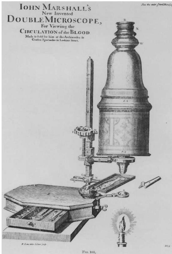
**Figure 1.** John Marshall's double microscope for viewing the circulation of the blood (from Harris's *Lexicon Technicum*, 1704, Figure 103, and W.B. Carpenter, *The Microscope and Its Revelation*. 7th ed. London: J & A Churchill, 1891;135-8.
