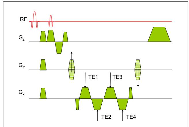
**Figure 3 Field-Mapping Pulse Sequence**
